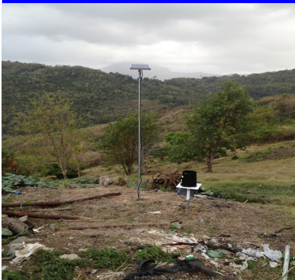
Rainfall logger and solar panel
