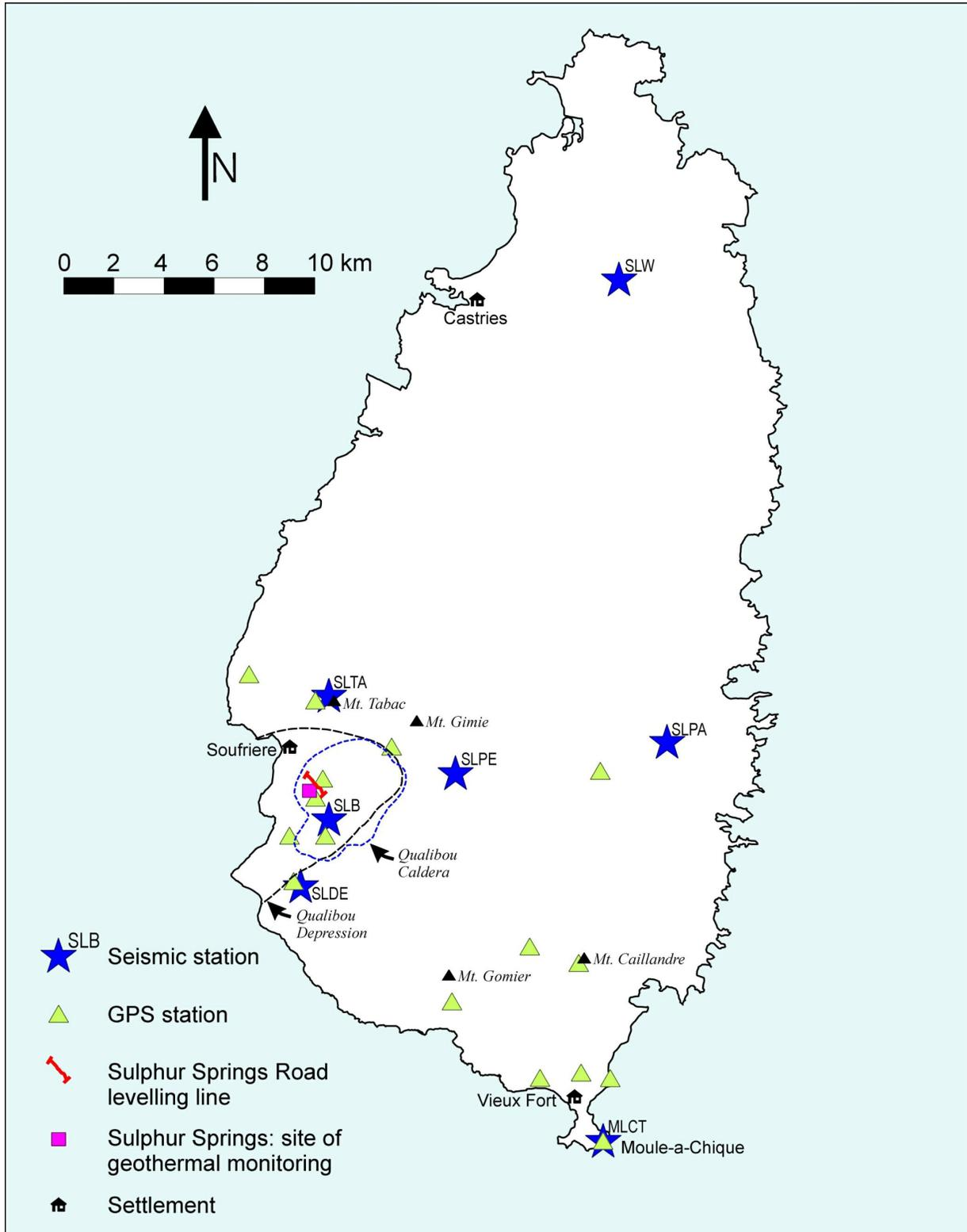
Figure 8: Volcano monitoring network in St Lucia. The base stations for both seismic and GPS sub networks are located at Moule-a-Chique.
