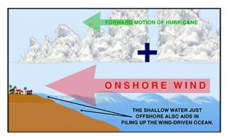
The main force creating the storm surge at the time the centre of the hurricane or tropical storm makes landfall is the wind driving the ocean ashore. The ocean creates frictional drag for the wind and therefore piles up against the coastline. Source: <u>http://www.hurricanetrack.com/ncstormsurae/srainf.html</u>
