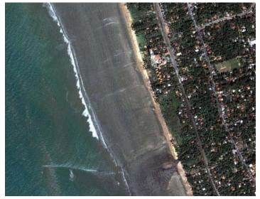
Sri Lanka, 26<sup>th</sup> December 2004 Image shows "drawback" or withdrawal of water exposing ~150 meters of temporary beach. Photo: <u>www.digitalglobe.com</u>
