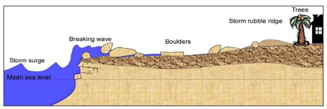
The calculation of setbacks for permanent structures on coastlines needs to be site-specific. The assessment of waves and associated boulders and debris encroachment inland can be used to assist in assigning site specific setbacks for shoreline construction. Diagram courtesy: Rowe, D-A., Khan, S.A. & Robinson, E., The University of the West Indies Marine Geology Unit.
