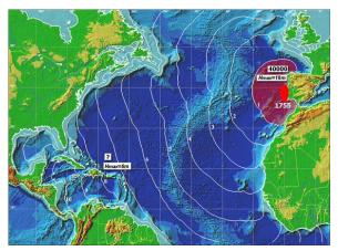
Tsunami travel time chart for the 1755 Lisbon tsunami. Solid ellipse marks position of the earthquake source. Red color shows the area within 1-hour propagation time. Source: <u>tsun.sscc.ru/TTT\_rep.htm</u>
